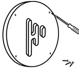
Align the holes then screw the nails into the drywall anchors using a screwdriver.
