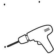
Make a hole on each mark using a drill with a 1/8" (6mm) drill bit.
