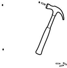
Tap the drywall anchor in the hole with a hammer.
